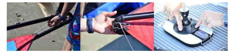
Feed outhaul through clew, pull to secure. Secure mast base using rubber supplied. Mast foot screws into recessed brass nut.
