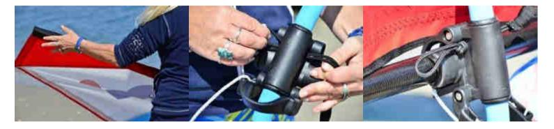
Fat head sail with single batten. Feed uphaul tie-off into uphaul hole, knot so as to secure in place.
