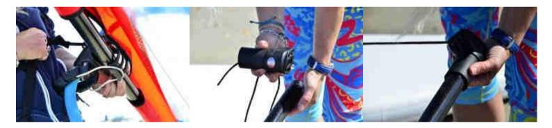
Approximate boom position within mast sleeve gap, relative to your height (shoulder). Slot in mast extension.
